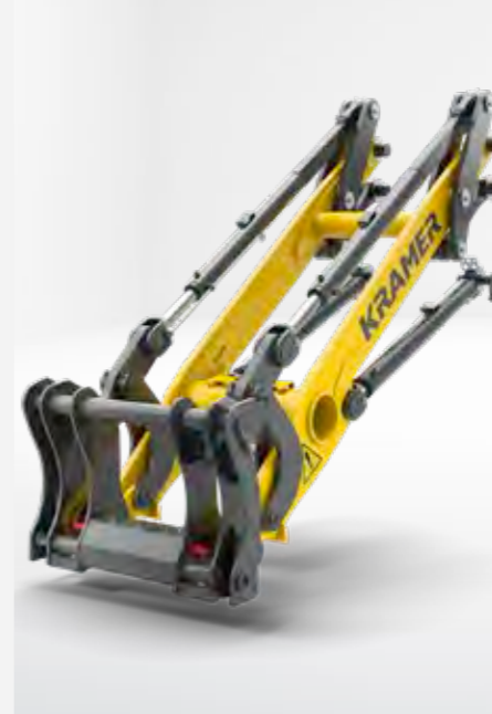
Industrial loader unit (P-kinematics) with Kramer quickhitch plate
