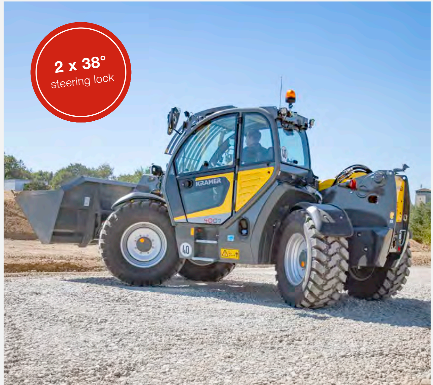
All-wheel steering: particularly manoeuvrable in tight spaces
